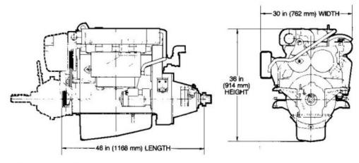
For complete dimensional information refer to installation drawing 2SA140 for Model 5042-4000, and 2SA246 for Model 5042-6000.
